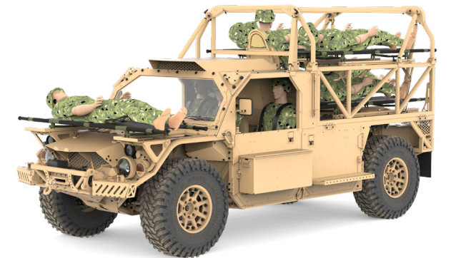
Tactical CASEVAC/Ambulance Kit Carries up to four litters and three operators in cab
