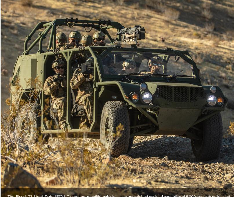
The Flyer® 72 Light Duty (F72-LD) ground mobility vehicle (F72-LD) is a lighterweight variant of the Flyer 72 base vehicle currently in operational use as the M1288 Ground Mobility Vehicle 1.1 (GMV 1.1) and XM1297 Army Ground Mobility Vehicle (A-GMV).
