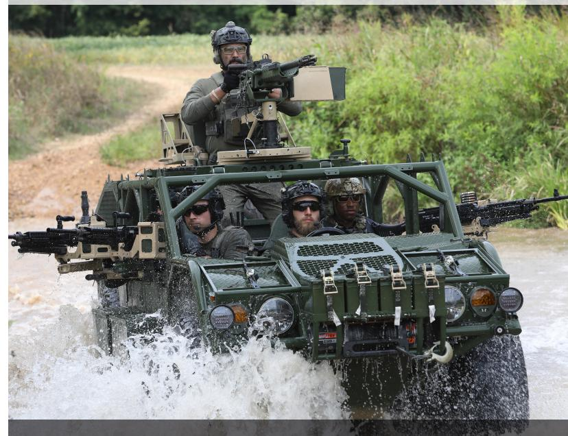
The Flyer® 60 ground mobility vehicle is a lightweight, highly mobile, air transportable platform capable of rapid configuration for a variety of mission needs. The Flyer® 60 meets all internal transport requirements for the V-22 Osprey and is also internally and externally transportable in the CH-53, C-130 and C-17 aircraft.
