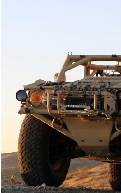
The Flyer<sup>®</sup> 60 ground mobility vehicle is a lightweight, highly mobile, air transportable platform capable of rapid configuration for a variety of mission needs. With a payload capacity of up to 4,100 pounds, the Flyer® 60 meets all internal transport requirements for the V-22 Osprey and is also internally and externally transportable in the CH-53, C-130 and C-17 aircraft.
