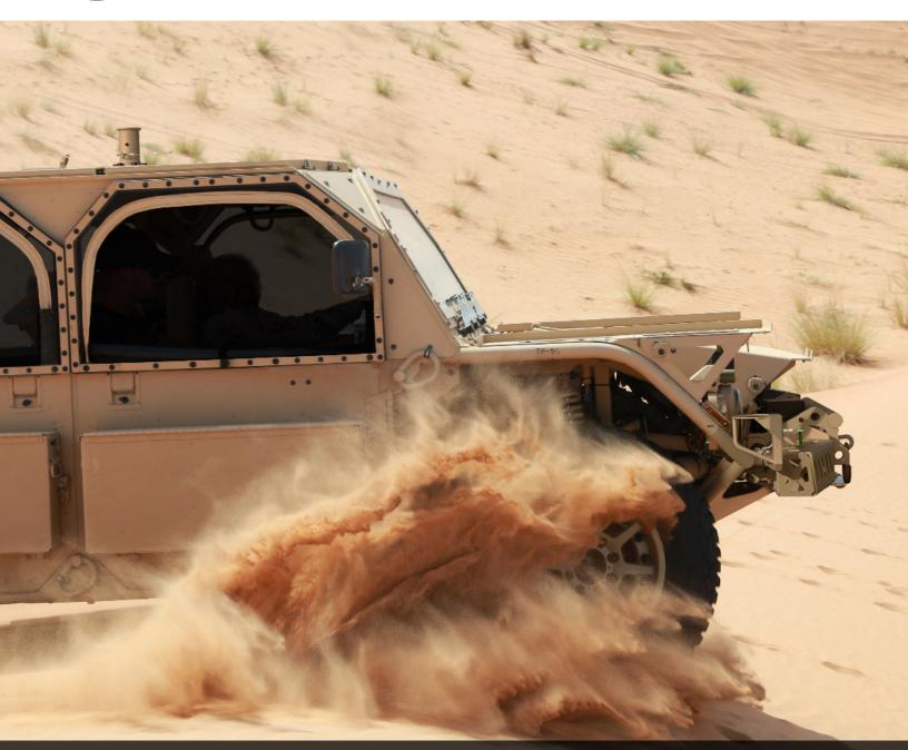
The Flyer<sup>®</sup> 72 - Heavy Duty (F72-HD) ground mobility vehicle, currently in production is a purpose-built, lightweight vehicle designed to meet complex mission sets. Selected by the U.S. Special Operations Command (USSOCOM) as the vehicle of choice for their Ground Mobility 1.1 (GMV 1.1) Program of Record, at 72" wide, it is capable of internal transport in the CH-47, CH-53, and C-130 aircraft.
