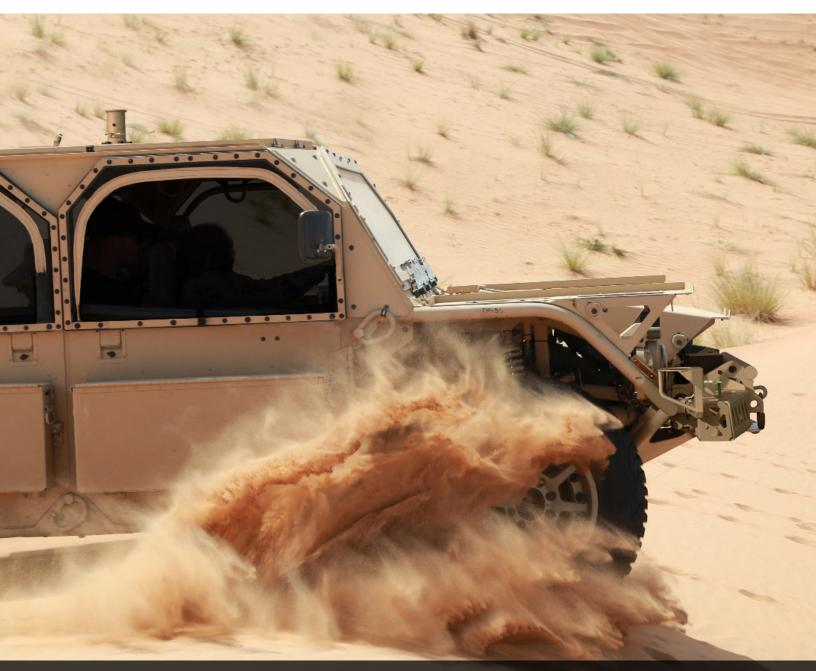
The Flyer® 72 - Heavy Duty (F72-HD) ground mobility vehicle, currently in production is a purpose-built, lightweight vehicle designed to meet complex mission sets. Selected by the U.S. Special Operations Command (USSOCOM) as the vehicle of choice for their Ground Mobility 1.1 (GMV 1.1) Program of Record, at 72" wide, it is capable of internal transport in the CH-47, CH-53, and C-130 aircraft.
