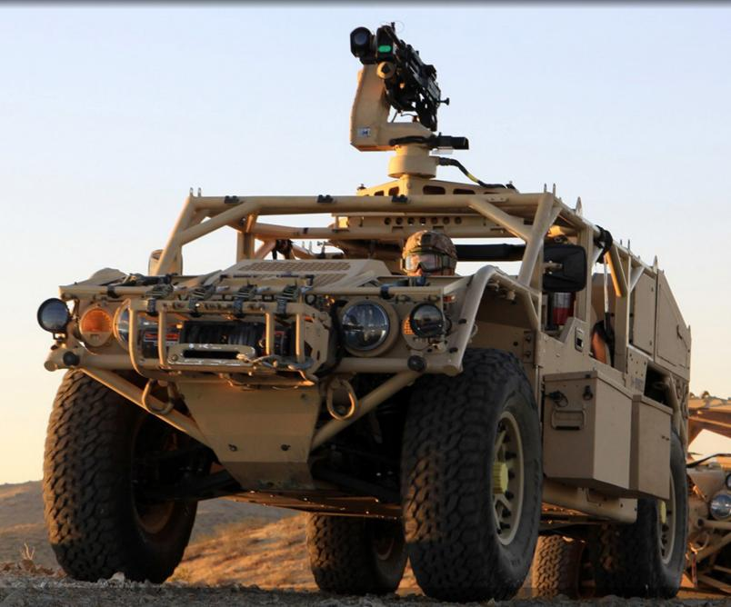
The Flyer® 60 ground mobility vehicle is a lightweight, highly mobile, air transportable platform capable of rapid configuration for a variety of mission needs. With a payload capacity of up to 4,100 pounds, the Flyer® 60 meets all internal transport requirements for the V-22 Osprey and is also internally and externally transportable in the CH-53, C-130 and C-17 aircraft.
