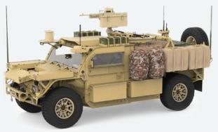
Manned or remote weapon station capable from 7.62mm to .50 caliber armament
