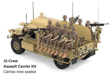
operators in cargo bed, three in cab
