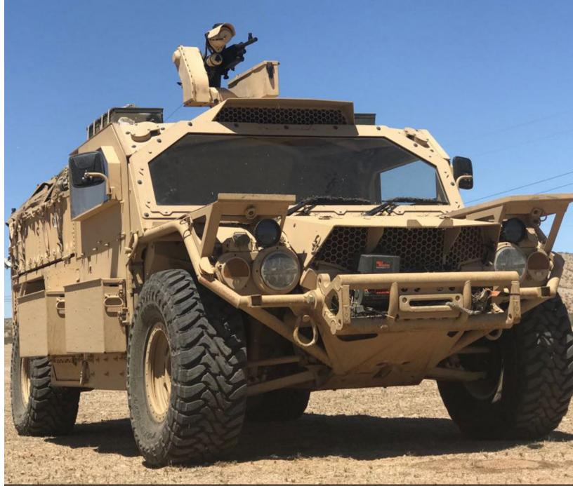
The Flyer® 72 Ground Mobility Vehicle - Utility (GMV-U) is an open cargo deck vehicle that is capable of supporting multiple mission kits. The GMV-U shares the same based design 90% component commonality with our USSOCOM's M1288 GMV 1.1 and US Army's M1297 A-GMV vehicles. The GMV-U can be used as a kit modification for either the M1288 or M1297 vehicles.
