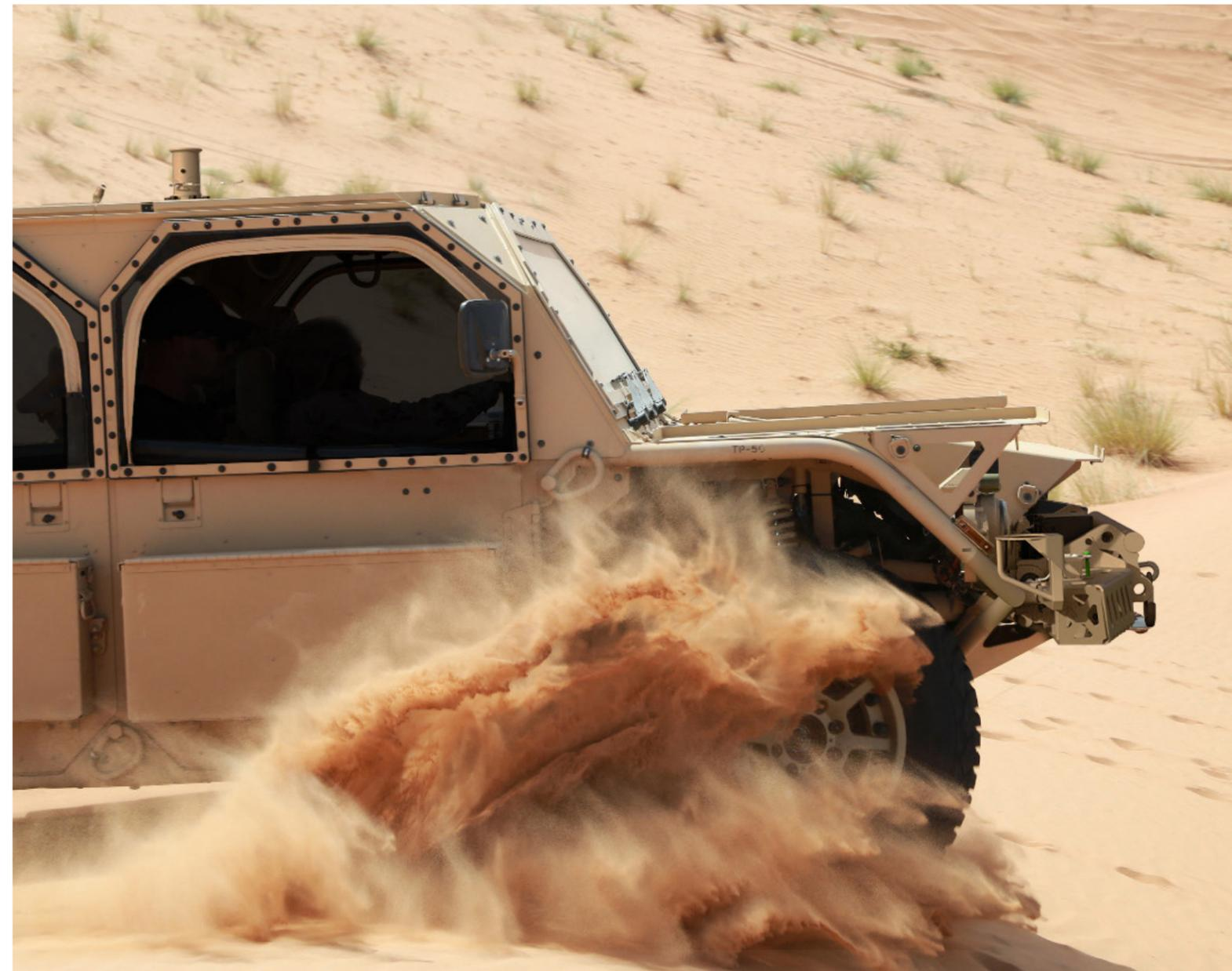
The Flyer<sup>®</sup> 72 is a non-developmental item, purpose-built, lightweight vehicle designed to meet complex mission sets. Selected by the U.S. Special Operations Command (USSOCOM) as the vehicle of choice for their Ground Mobility 1.1 (GMV 1.1) program, at 72" wide it is capable of internal transport in the CH-47 and C-130 aircraft.
